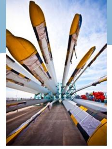
In addition to being highly engineered and sensitive, wind turbine blades are matched and balanced, and must be delivered to the job site in sets.
